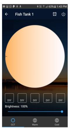
Device type "CCT" controls two channels independently. For example if you had 2 x XB2 tubes connected then you would be able to dim/brighten the two tubes independently.
