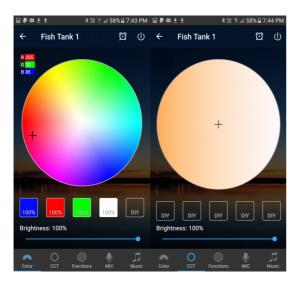
Device type "RGBWW" controls 5 channels independently, one screen to manage the 3 RGB channels just like device type RGB and a second screen to manage the fourth and fifth channels just like device type CCT, most commonly used on systems that have a mix of RGB leds and XB2 power leds with the power leds connected to the fourth and fifth channels.
